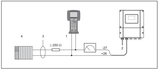
Fig. 36: Electrical connection of the HART handheld communicator: 1 = HART communicator, 2 = power supply, 3 = shield, 4 = other evaluation devices or PLC with passive input
