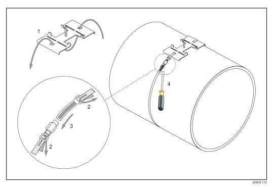
Fig. 12: Tensioning band installation for DN 250...4000
