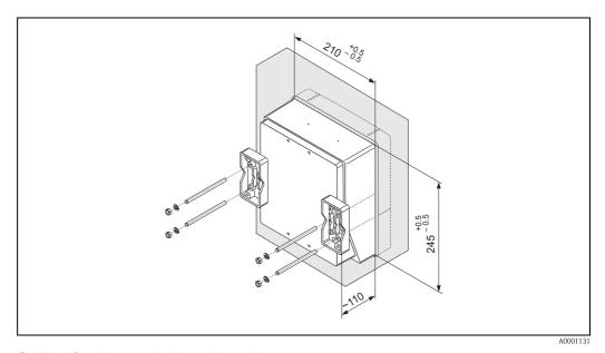
Fig. 31: Panel mounting (wall-mount housing)
