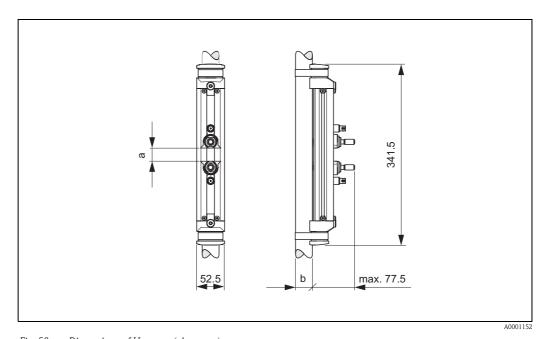
Fig. 58: Dimensions of U sensor (clamp-on)
