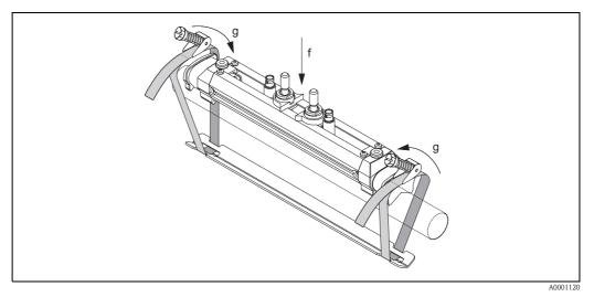
Fig. 20: Positioning the sensor and looping the tensioning bands
