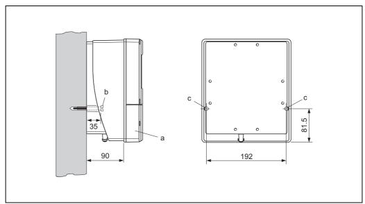
Fig. 30: Mounted directly on the wall
