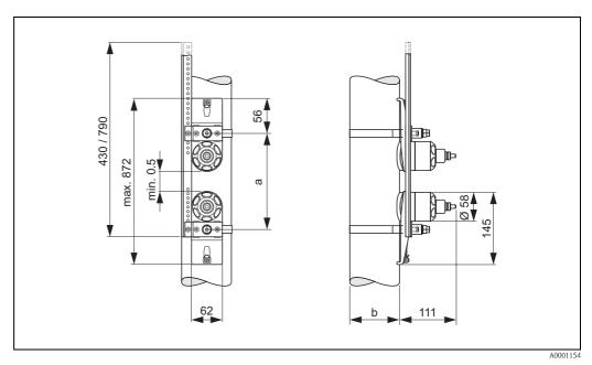
Fig. 55: Dimensions of P sensor (clamp-on) / (version: 2 or 4 traverses)
