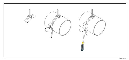
Fig. 11: Tensioning band installation for DN 50...200
