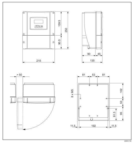
Fig. 54: Dimensions of wall-mount housing (panel mounting and pipe installation  $\rightarrow$  Page 33)
