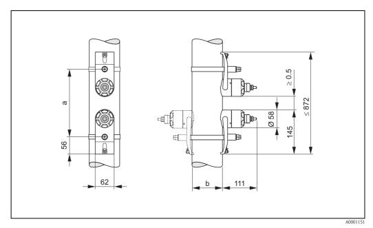
Fig. 57: Dimensions of W sensor (clamp-on)
