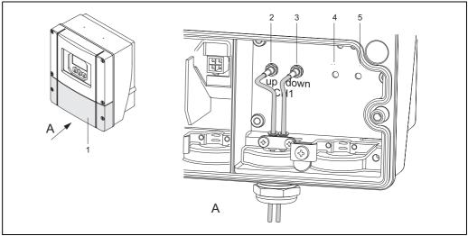
Fig. 33: Connecting the measuring system
