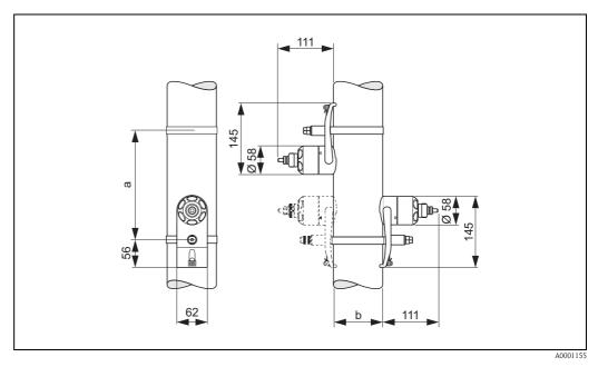
Fig. 56: Dimensions of P sensor (clamp-on) / (version: 1 traverse)
