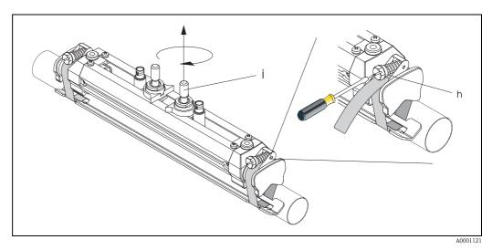
Fig. 21: Tightening the tensioning bands and the screw adjustment
