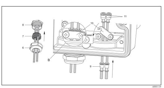
Fig. 34: Connection of the sensor connecting cable
