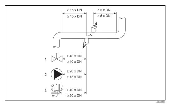
Fig. 9: Inlet and outlet runs (Insertion version)
