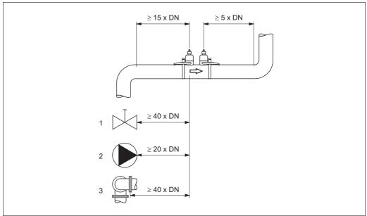
Inlet and outlet runs (clamp-on version) 1 = Valve; 2 = Pump; 3 = Two pipe bends in different directions
