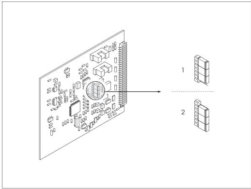
Fig. 47: Current output configuration (I/O board)
