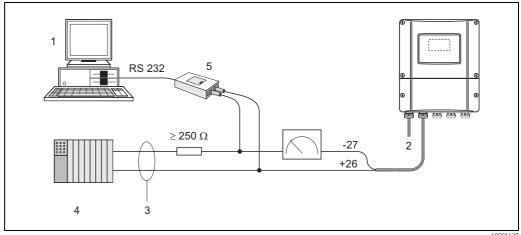
Electrical connection of a PC with operating software I = PC with operating software, 2 = power supply, 3 = shield, 4 = other switching units or PLC with passive input, 5 = HART modem, e.g. Commubox FXA 191
