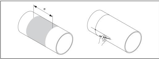
Fig. 24: Installing the measuring sensors, steps 1 and 2
