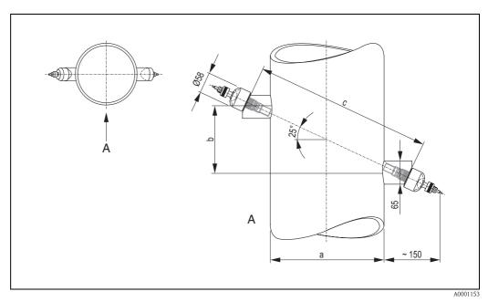
Fig. 59: Dimensions of W sensors (Insertion version)
