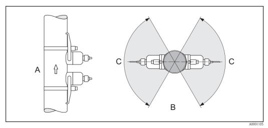
Fig. 7: Installation position (A = vertical, B = horizontal, C = recommended installation range max. 120°)
