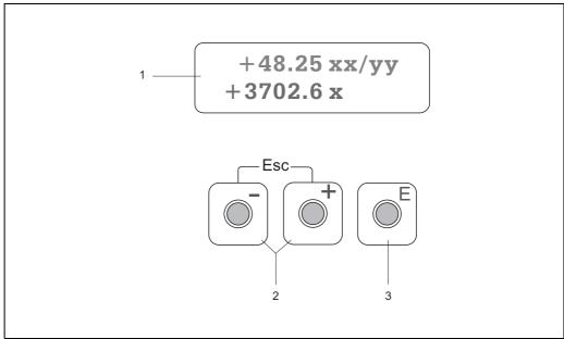
Fig. 41: Display and operating elements
