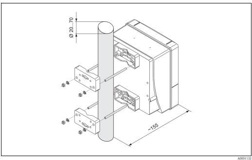
Fig. 32: Pipe mounting (wall-mount housing)
