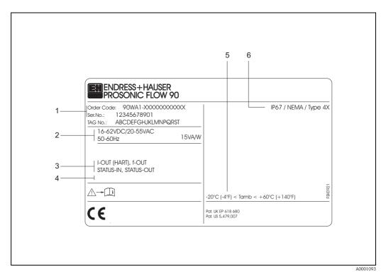
Fig. 1: Nameplate specifications for the "Prosonic Flow 90" transmitter (example)
