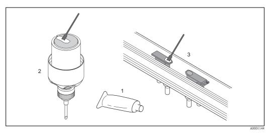
Fig. 48: Application of the coupling fluid
