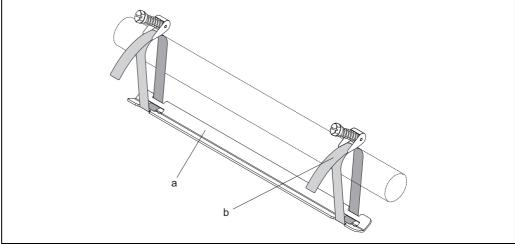
Fig. 18: Preparing sensor installation with retaining vee
