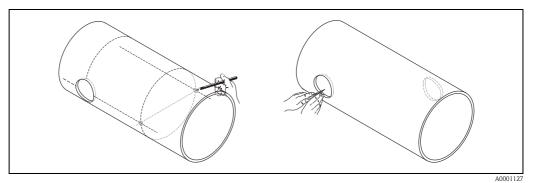
Fig. 27: Installing the measuring sensors, steps 7 and 8
