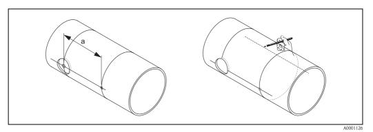
Fig. 26: Installing the measuring sensors, steps 5 and 6
