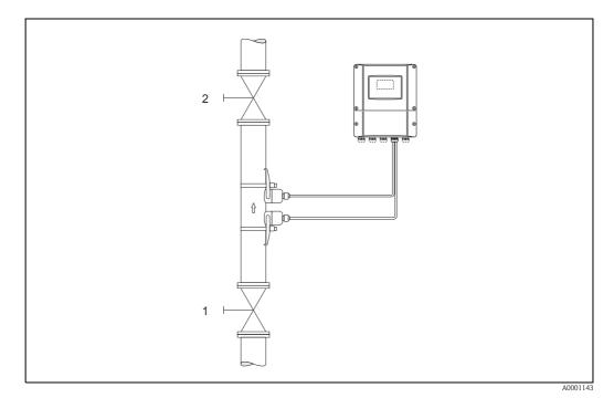
Fig. 46: Zero point adjustment and shut-off valves
