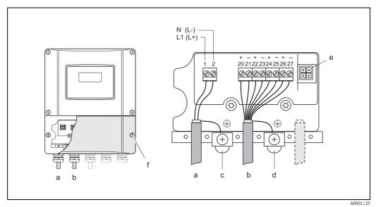
Fig. 35: Connecting the transmitter (wall-mount housing) Conductor cross-section: max. 2.5 mm<sup>2</sup>
