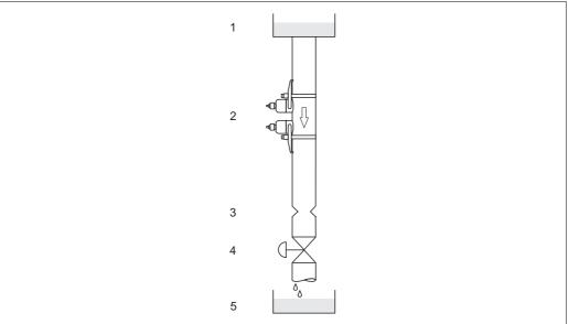
Fig. 6: Installation in a down pipe 1 = Supply tank; 2 = Measuring sensors; 3 = Orifice plate, pipe restriction; 4 = Valve, 5 = Filling tank
