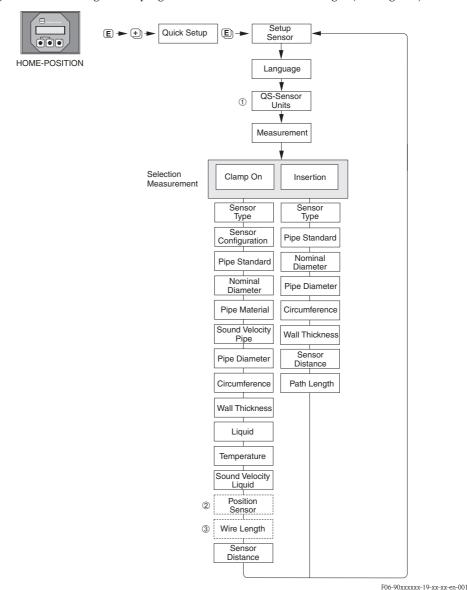
Fig. 44: "Quick Setup" menu for sensor installation
