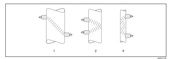
Fig. 10: Sensor arrangement (clamp-on)
