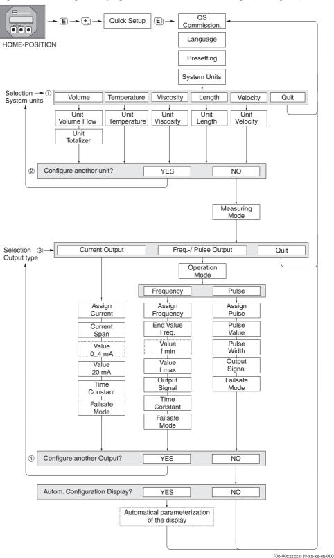
Fig. 45: "Commissioning" Quick Setup for rapid configuration of important device functions For an explanation of points  $\bigcirc - \bigcirc$ : see next page
