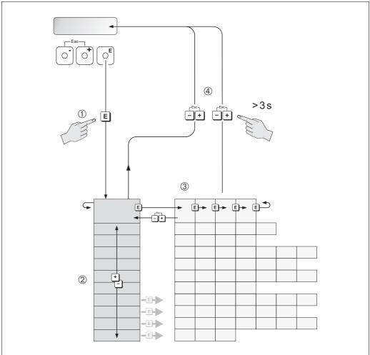
Fig. 42: Selecting functions and configuring parameters (function matrix)
