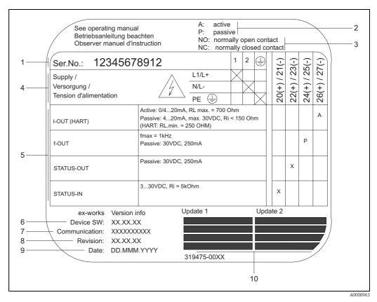
Fig. 4: Nameplate specifications for Proline transmitter (example)
