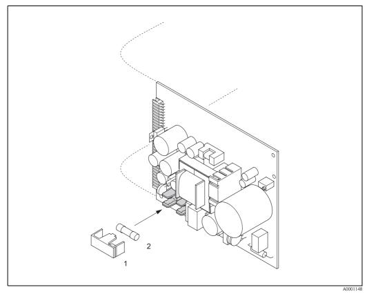
Fig. 52: Replacing the device fuse on the power unit board
