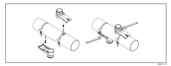
Fig. 16: Installing the sensor holders
