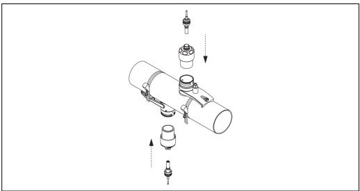
Fig. 17: Installing the sensors and the sensor connectors
